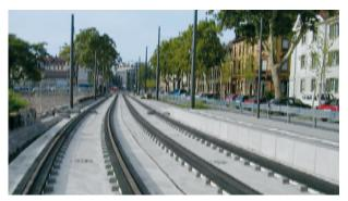
**POWER THROUGH PEACE AND QUIET** Green track chamber elements prevent the vegetation from growing completely up to the rails. A simultaneous effect is reduction of airborne noise emission.
