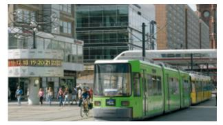
**RHEDA CITY: THE SAFE WAY TO GO** As a ballastless track system, RHEDA CITY can be optimally integrated into traffic flow: trams, buses, cars, and pedestrians all share the same trackway. The system can be covered with asphalt or other paving material, as required.
