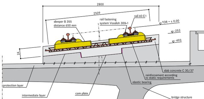
Connection of the track concrete layer with the bridge structure by means of negative cam plates
