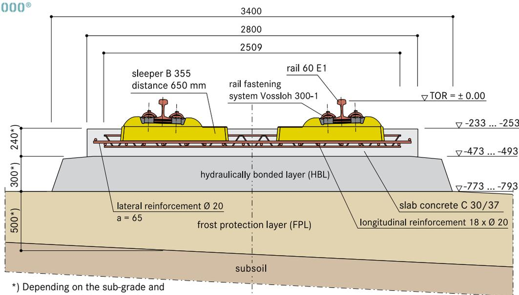
**RHEDA 2000® is a flexible system that can be individually adapted to the specific requirements and the individual constraints of each project.** The basic system structure, however, always consists of modified bi-block sleepers which are securely and reliably embedded in a monolithic concrete slab. Highly elastic rail fastenings are essential to achieve the vertical rail deflection required for load distribution and for smooth train travel.
