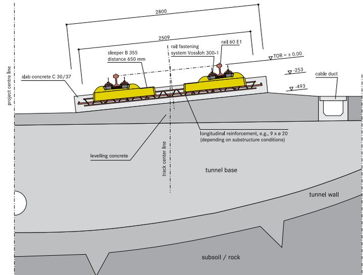
Track concrete layer, installed on levelling concrete
