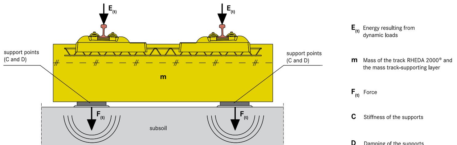
Application of the single-mass oscillator principle in the RHEDA 2000® track type on a mass-spring system
