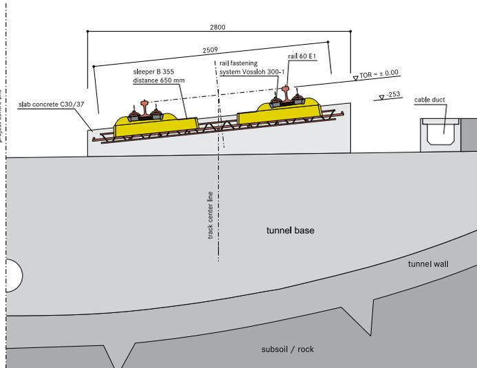
Track concrete layer, installed on tunnel-floor fill
