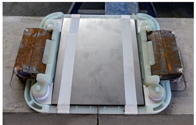
Figure 5: Intermediate pad with sensor at rail seat
