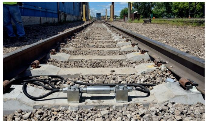
Figure 4: sensors on top of the sleeper center
